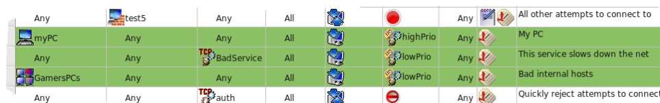
Figure 1: Excerpt from my policy that shows the traffic classification rules. My PC is allowed to suf fast while all GamersPC are slowed down. The same fate happes to traffic the a bad service.
